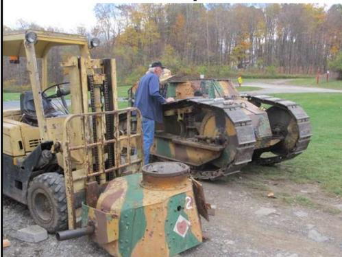
The planes are the stars of the show, but everyone seems to love the M1917 Tank. After years with, of all things a Chevette engine, the car crew is reinstalling an overhauled Budda. That means it will actually be able to turn reliably, run forward and reverse.
